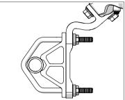
Correct orientation of the Large Pole Mount bracket is shown below, for pole diameter span: 39 - 55 mm.
