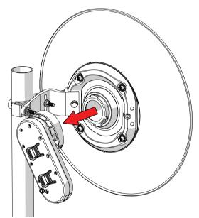
Model STD-24-UM shown. Installation instructions are identical for other StarterDish<sup>™</sup> models. Antenna dimensions may differ.
