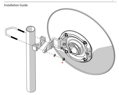
\* Optional: Surface treated M6 Nuts protect the bracket from galling. If you use M6 nuts without surface treatment, use anti-seize thread lubricant.
