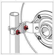
$Model \ STD-24-UM\ shown.\ Installation\ instructions\ are\ identical\ for\ other\ Starter Dish^{\text{\tiny M}}\ models.$  Antenna dimensions may differ.
