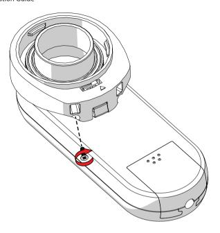
Use Phillips Screwdriver when assembling the adaptor.
